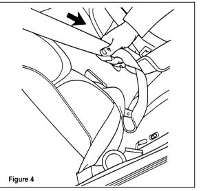
Setting the retractor to automatic locking mode
